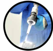
Dry Ice Blasting
